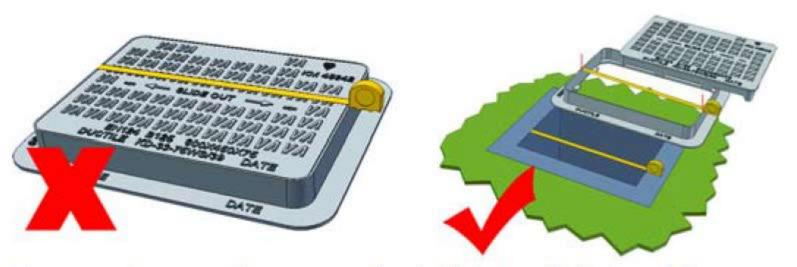
Many customers will measure the 'visible' or 'lid' size of the cover which is larger than the clear opening (hole size) often stating 650x550mm or 25"x18" (inches) these usually all have a 600x450mm clear opening dimension. Manhole covers must be larger than the clear opening (hole) to prevent them falling into the chamber.
